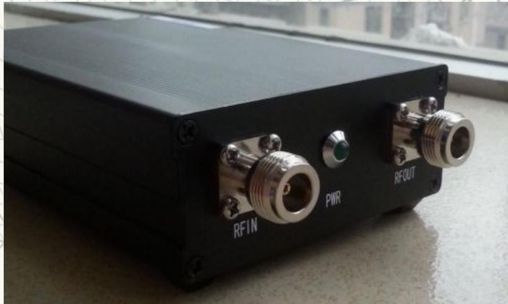
NWT4000-2 35M-4.4G sweep simple spectrum analyzer generator
